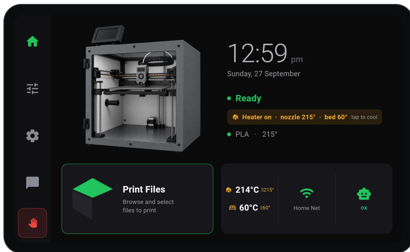
Figure 77 Heaters left on after a job. Tap the amber line to switch them off.
